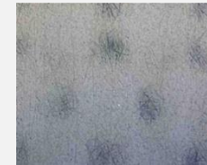
Surface when surfacing film used
