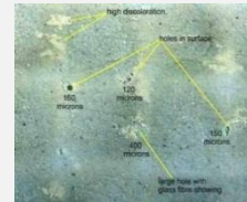
Surface without surfacing film
